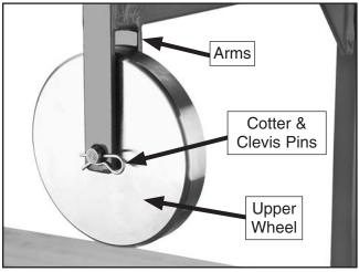
Figure 8. Upper wheel installed.
